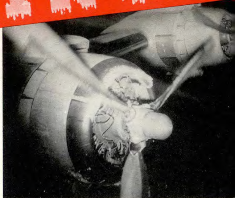
C-54 engine and B-29 nose show ice formed in flight.
