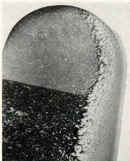
This propeller tip shows how ice builds up on leading edge.
