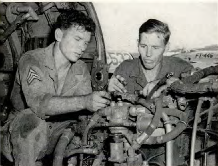
Mechanics work around the clock to keep jet fighters ready for daily missions. Above, Sgts. W. P. Holloway and H. B. Huckabee remove oil filter. Below, Sgt. W. L. Alldridge changes machine gun.
